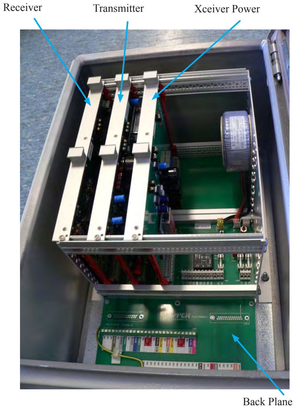
Fig. 10.1 PCB positions in Transceiver Unit
